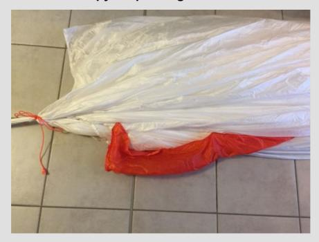
Push back the half side of the canopy underneath, so that the red marking of the front tip, that shows the flight direction, is closed to you.
